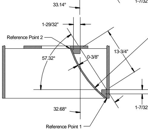
Note: Horn Flare Radius Center point location can be found from the two reference points.
