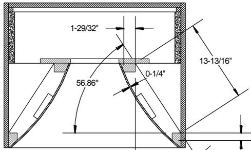
Item 12 shown in the parts drawing is not an exact fit as these drawings show. Choose the flare thickness you intend to use and cut the brace to these dimensions for a more accurate fit. A full size brace drawing for both 1/4" and 3/8" flare thickness is included that may be used as a pattern.
